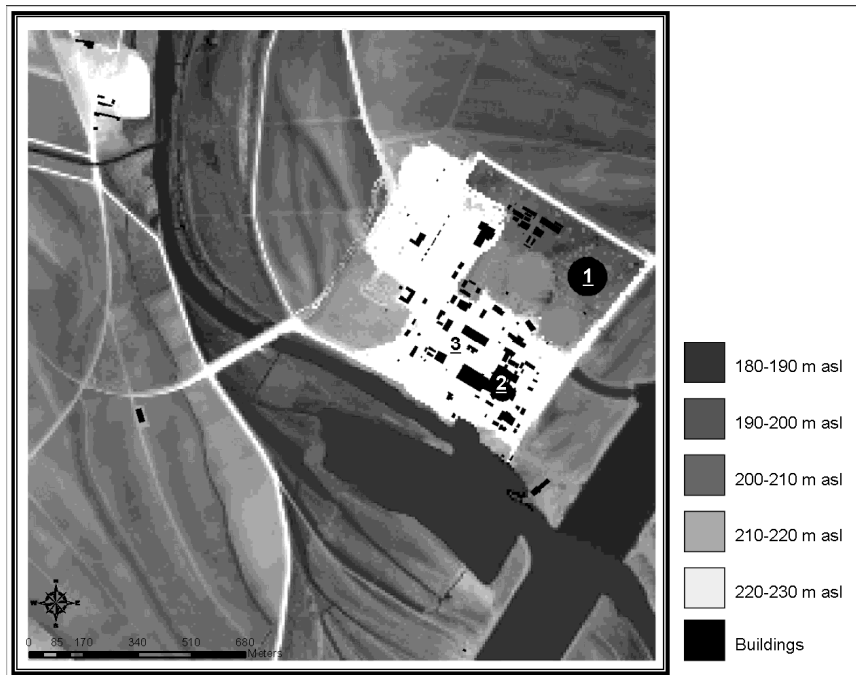
Figure 4. Exemplary map for a thermal power plant. (1) The cooling tower is in a flooded area, the cooling tower pond is already flooded to avoid its floating. (2) The production unit is in a non-flooded area as well as (3) the offices and shops, no damages are expected.
